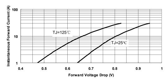
Fig.3-Typical Forward Voltage Drop Characteristics
